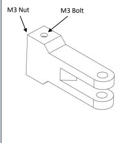
Note: Only tighten enough to engage the nut.
